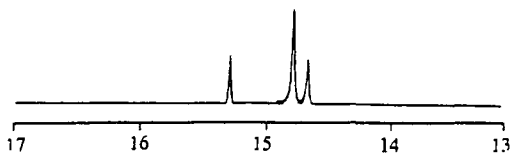
Figure 9. Portions of the ^1\text{H} NMR spectra of the self-assembled aggregates showing the resonances associated with the hydrogen-bonded isocyanurate protons ( \text{CDCl}_3 , 500 MHz).
